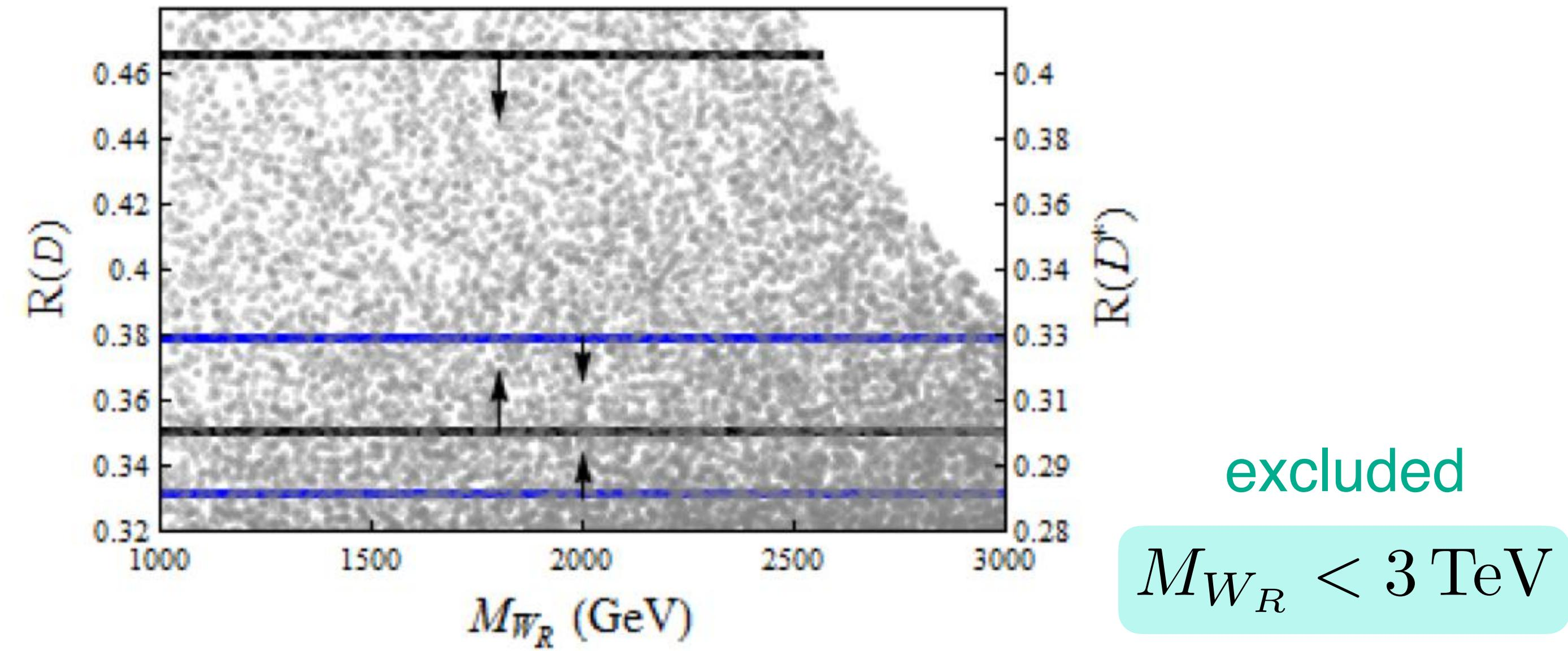
Figure 4:  $R(D, D^*)$  scatter-plot is shown by varying  $g_R$  and  $M_{W_R}$ . The boundaries of  $R(D)$  and  $R(D^*)$  anomalies are shown by black and blue lines respectively. We show  $1\sigma$  allowed regions.
